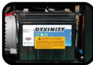
STEP 2. Connect the battery before starting.
