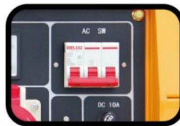
STEP 3. Turn the circuit breaker off.
