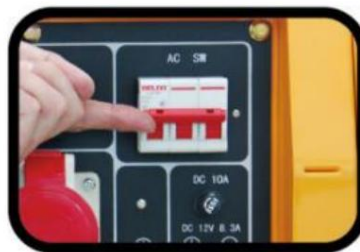
STEP 11. Turn the circuit breaker on.
