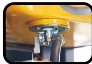
STEP 6. Turn the fuel switch on.
