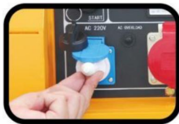
STEP 10. Connecting the load.
