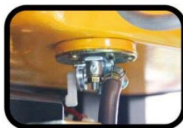
STEP 6. Turn the fuel switch on.
