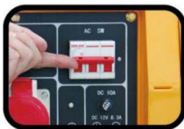
STEP 11. Turn the circuit breaker on.
