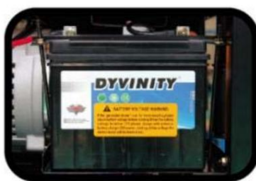
STEP 2. Connect the battery before starting.
